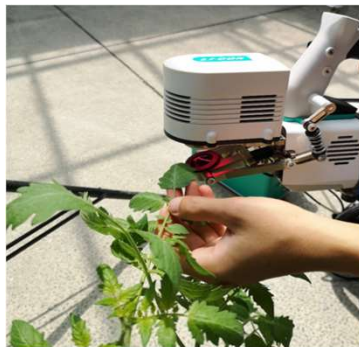
Demonstration of environmental, physiological and NIR spectrum data collection by portable photosynthesis system LI-6800 (left) and spectroradiometer MS-720 (right).
